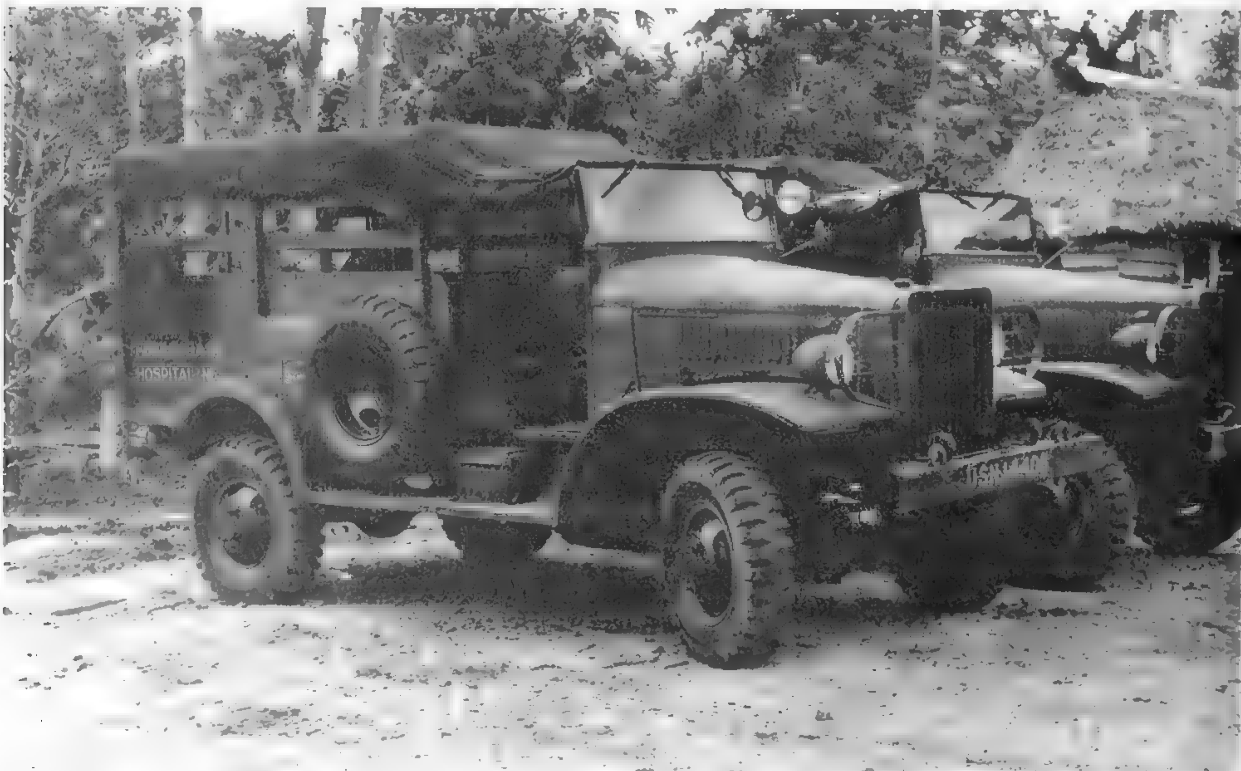
Ambulance versions of the M-1-4 had canvas-covered collapsible bodies built by Boyertown. They more closely resembled cargo trucks than they did ambulances. (Photo courtesy of the Military History Institute)
